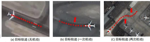
((a) target trajectory (no maneuvering); (b) target trajectory (one maneuver); (c) target trajectory (two maneuver))
